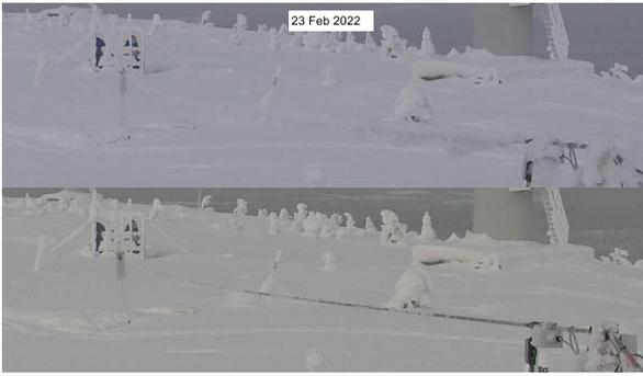
Figure 6. Before and after images from series of 4 successive ice dropper launches on 23<sup>rd</sup> of February. Ice is partially removed and the cable is exposed.
