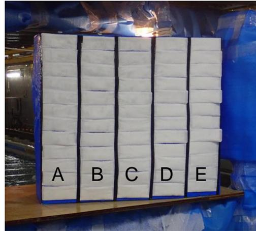
Fig. 7 A measurement of the distribution of urea-doped spray water.
