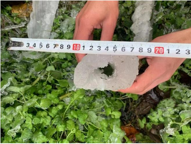
Fig. 1 The residual ice after ice-shedding.
