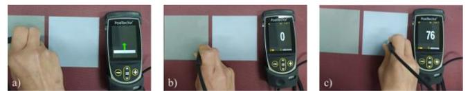
Fig. 2 Step followed for the measurements of the coating's thickness.
