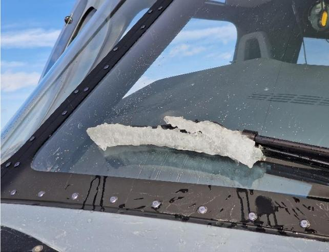
Fig. 1. Iced windshield wiper after encountering severe icing near Alta on the 19<sup>th</sup> of April. Photo by Eirik Mikal Samuelsen.
