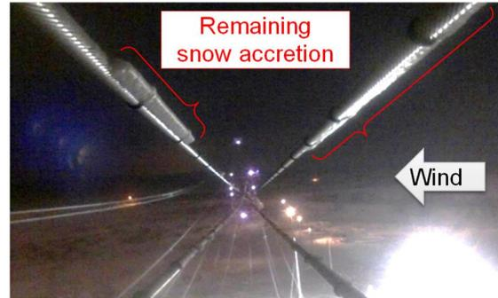
Fig. 1 Example of photograph of wet snow accretion just before snow shedding.
