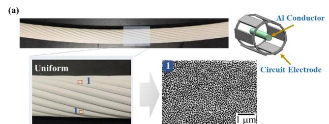
Fig. 2 Macro and micro morphology of Y-AAO conductor and ring electrode.
