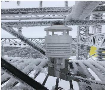
Fig.4 Six elements meteorological sensor
