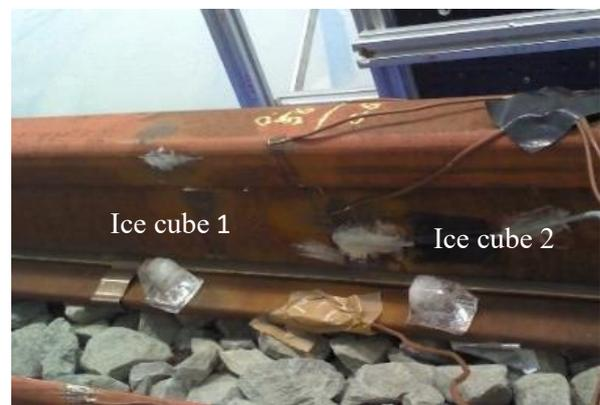
Figure 3. Location of ice cubes on the rail for de-icing study.
