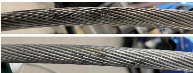
Figure 8. Scratches on the cable after test campaign.
