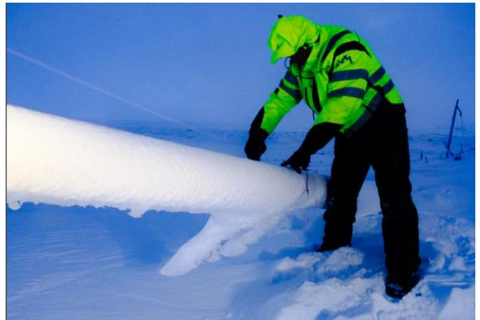
Fig. 18 Large ice diameter. Accumulation is influenced by drifting snow near the ground.
