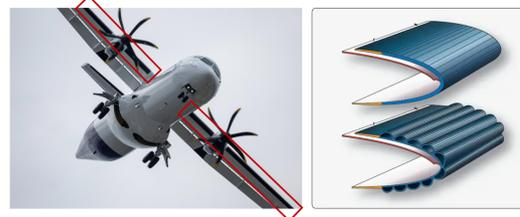
Figure 6: Pneumatic de-icing solution - Safran Aerosystems / Boots system closeup
