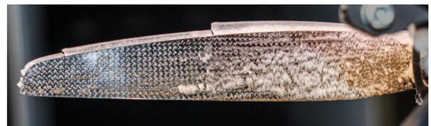
**Figure 3:** Ice accretion on a RPAS propeller after several ice-shedding events, creating “steps” on the leading edge.
