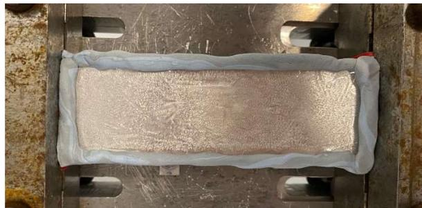
Fig. 4 Confined region using a pressure-sensitive adhesive to prevent water from slipping.
