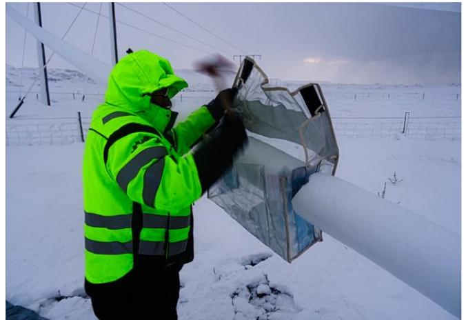
Fig. 17 Measurement of ice mass and ice density in KS1. Ice mass 14.8 kg/m and density 0.68 g/cm<sup>3</sup>.
