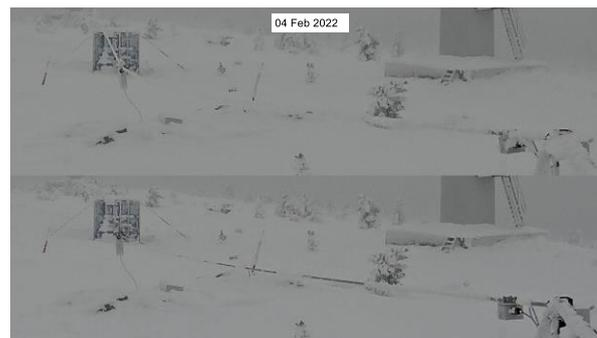
Figure 4. Before and after images from series of 4 successive ice dropper launches on 4<sup>th</sup> of February. Ice is partially removed and the cable is exposed.
