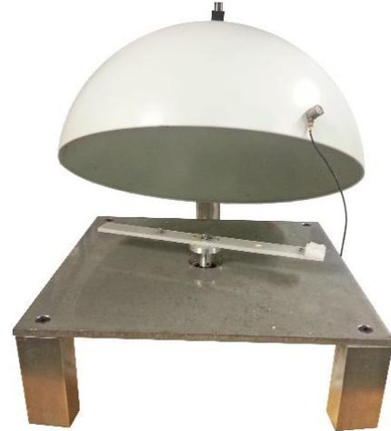
Figure 3. Centrifugal ice adhesion tester (CAT) at Tampere University, Ice Laboratory.
