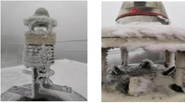
Fig. 11 Ultrasonic in icing environment
