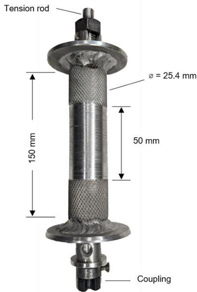
Fig. 1 Multi-component cylinder used for fabricating tubular ice tensile specimens.
