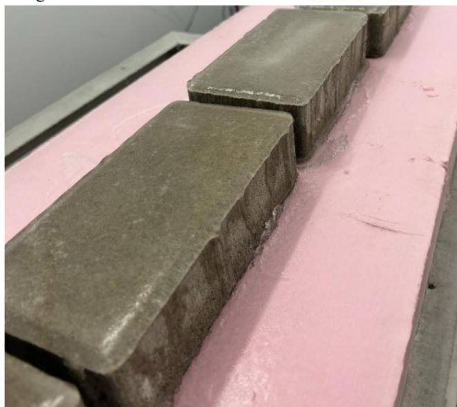
Fig. 2: Concrete samples after icing in the cold room
