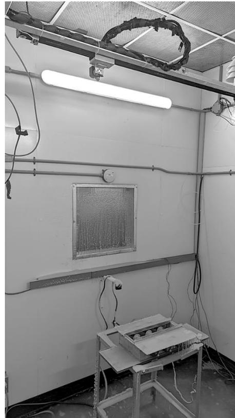
Fig. 3 Freezing drizzle icing experimental setup
