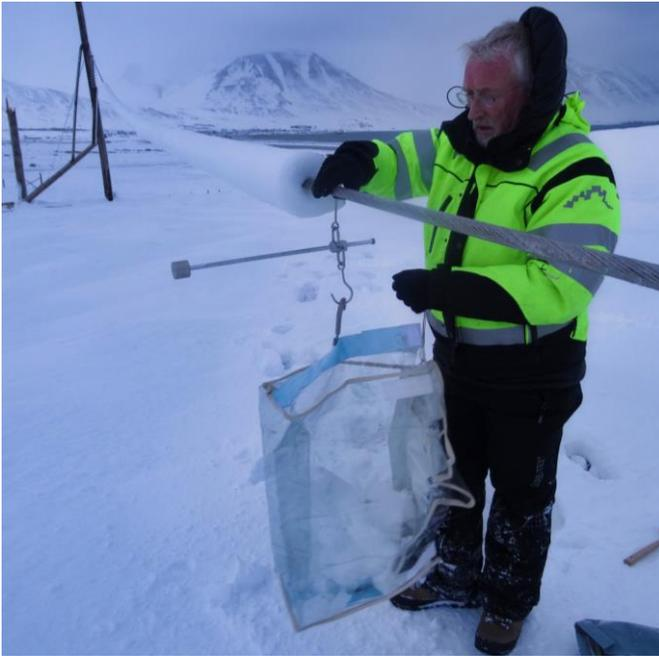
Fig. 8 Measurement in DA1. Ice mass = 16.8 kg/m and density = 0.76 g/cm<sup>3</sup>.
