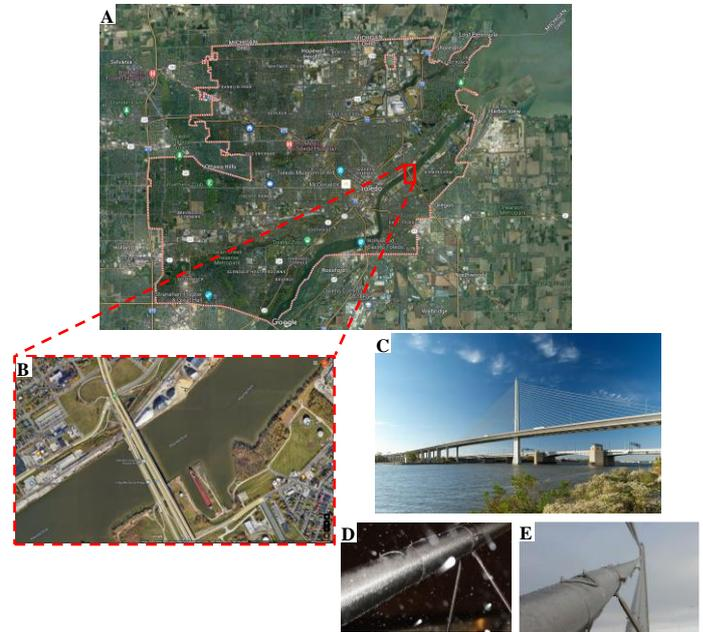
Fig. 1 A) Google map images of the city of Toledo in Ohio showing the location of the VGCS bridge, B) a zoom-in image of the VGCS bridge, C) an image of the VGCS bridge crossing the Maumee River [image source: FIGG Bridge Group], and D&E) ice accreting on the bridge cables during the 2011 ice event.
