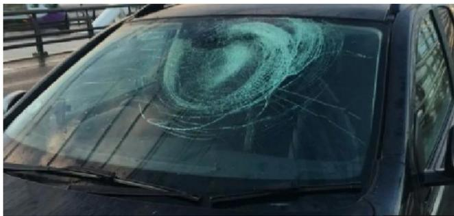
**Figure 2: Windscreen damaged by an ice piece falling from the towers/stay cables of the Queensferry Crossing bridge. Photo: Graeme Stevenson**
