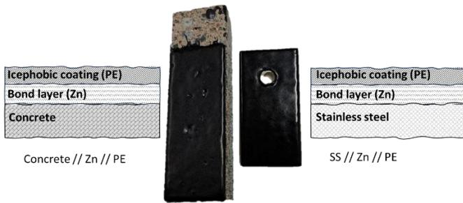
Figure 3 Digital images of coatings on concrete and SS substrates together with their schematics of the structure.
