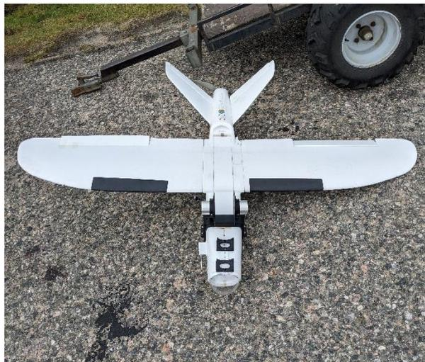
Fig. 3 Photo taken of the X-UAV Talon equipped with the UAV cloud particle sensor during the measurement campaign in Pallas.
