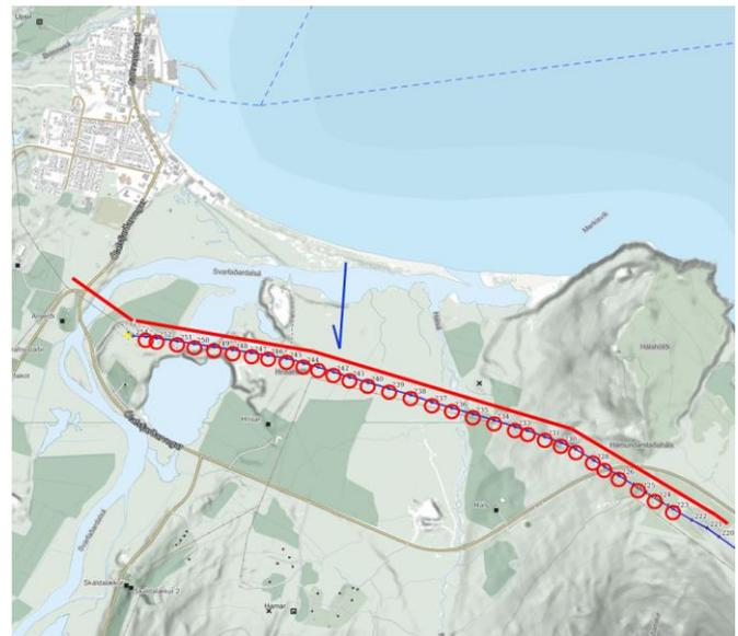
Fig. 5 The iced section of DA1, red circles show broken poles. Blue arrow shows direction of accumulation on poles.
