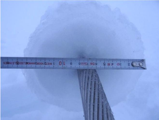
Fig. 9 Measurement of ice diameter 14 cm.
