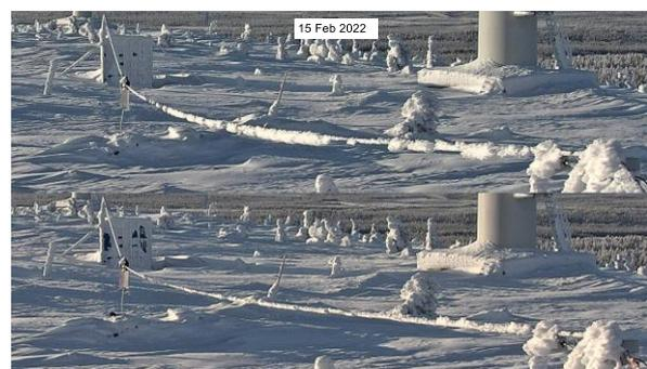
Figure 5. Before and after images from series of 4 successive ice dropper launches on 15<sup>th</sup> of February. Cable is not exposed but large chunks of ice was shed.
