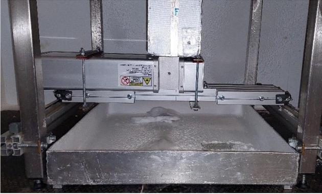
Figure 1. HiWatch HR2 diagnostic camera in water droplet measurement position under IWiT at Tampere University, Ice Laboratory.
