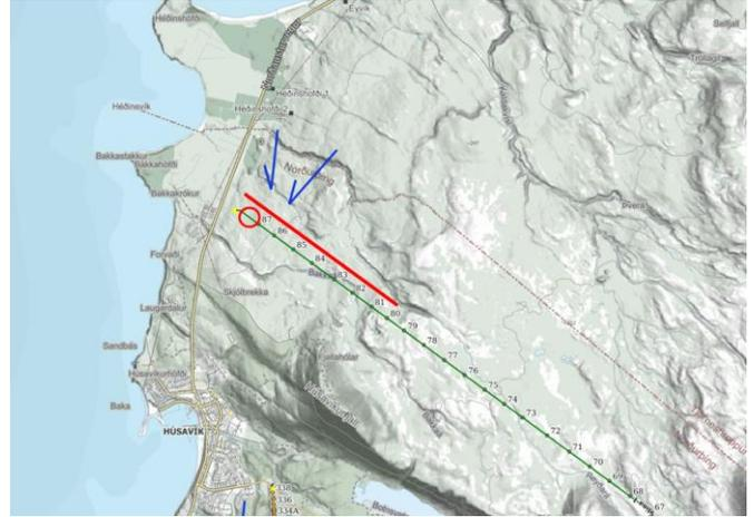
Fig. 11 The iced section of TR1, red circle, shows a damaged conductor. Blue arrows show the direction of icing on towers.
