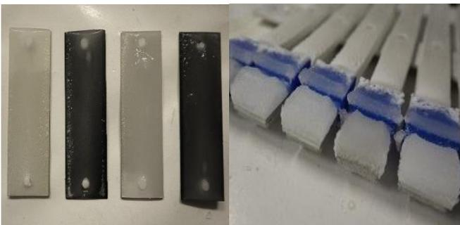
Figure 2. Heat plate samples on the left and samples for CAT testing with the masks after ice accretion on the right.
