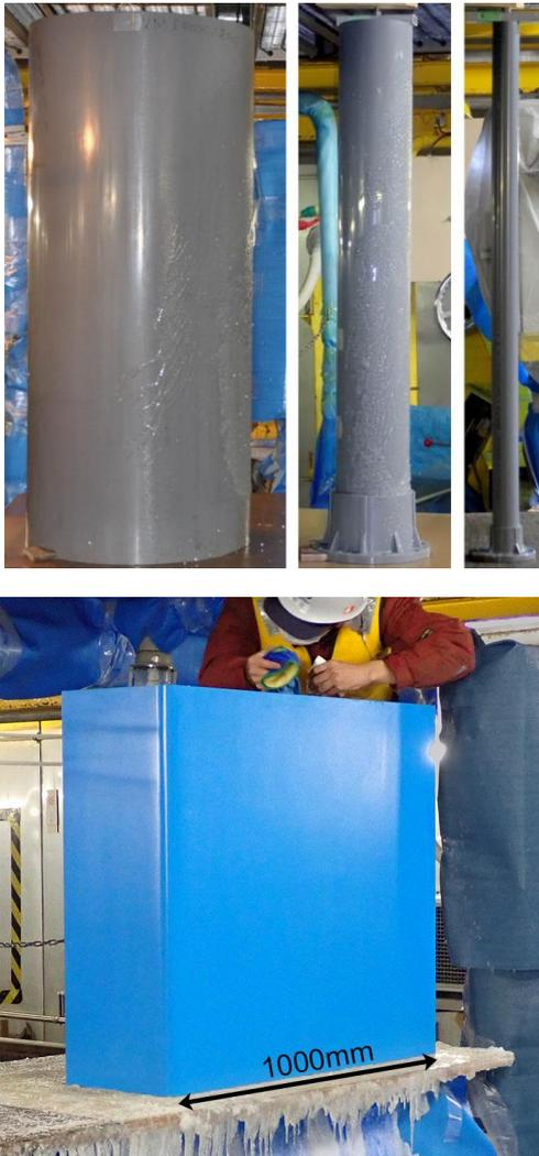
Fig. 2 Cylindrical and flat-plate specimens. Diameters of cylindrical specimens are 520 mm, 165 mm, or 60 mm.
